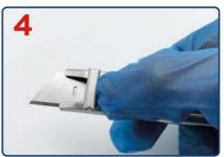
CAREFULLY FOLD THE TOP OF THE KNIFE CASING BACK DOWN ONTO THE BLADE. THE BLADE SHOULD BE ALIGNED WITH THE KNIFE AND WILL THEN MOVE FREELY.
